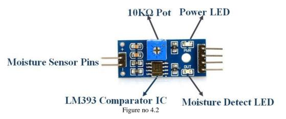
LM393 Comparator IC is used as a voltage comparator in this Moisture sensor module. Pin 2 of LM393 is connected to Preset ( $10K\Omega$  Pot) while pin 3 is connected to Moisture sensor pin. The comparator IC will compare the threshold voltage set using the preset (pin2) and the sensor pin (pin3).
